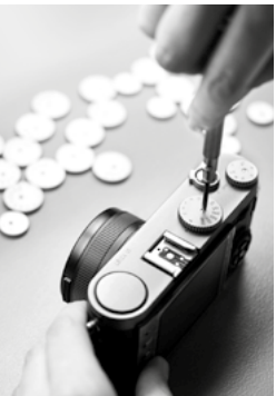
Leica X camera: fitting the shutter speed dial.
