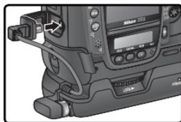
5 Pass the cable over the guide on the BL-2 battery-chamber cover.
